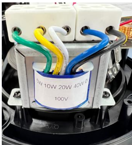
Fig. 2. CS7 wire connection (with transformer TF-100)
