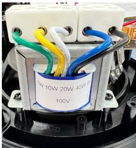
Fig. 2. CS7 wire connection (with transformer TF-100)
