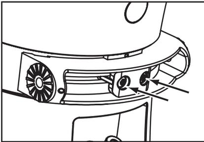
Figure 7. Qi 45EW Angle Adjustor screws
