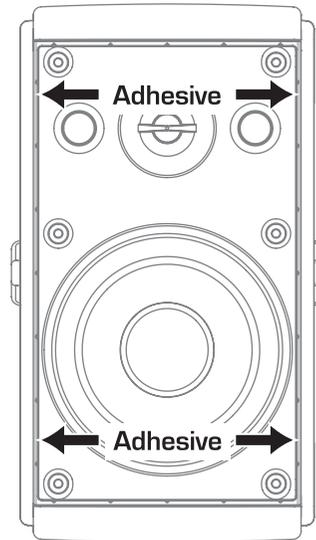
Figure 12. Positioning of adhesive strips before replacing grille
