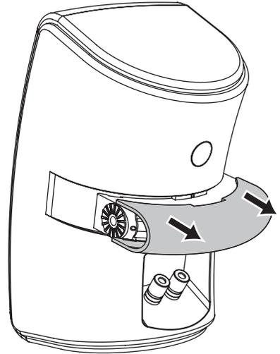
Figure 6. Qi 45EW removing angle adjustor cover
