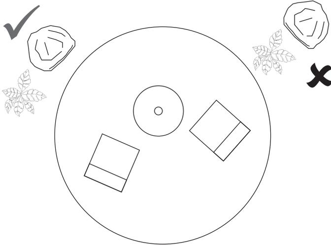
Figure 2. Position speakers clear of acoustic obstructions
