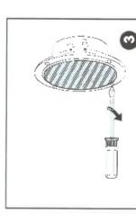
Screw down each of the four Phillips head screws. The locking tabs will swivel into place and secure the unit to the rear surface of the drywall. Put in the strips of adhesive to secure the grille.
