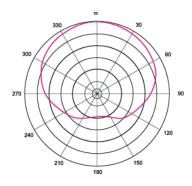
Directivity: Uni-directional Output connections: XLR (3-pin) Frequency Response: 50Hz - 14 KHz
